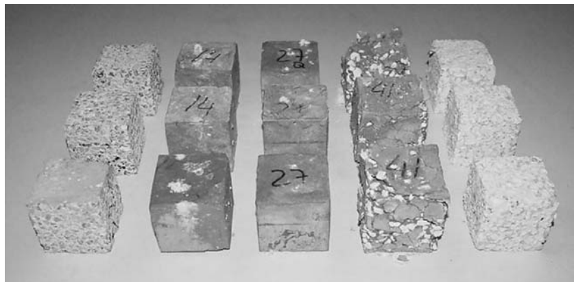
Fig. 1. Visual appearance of the specimens in sulfuric acid solution (a) OPC concrete with granitic aggregates; (b) mine waste paste (c) mine waste with granitic aggregates (d) mine waste with limestone aggregate (e) OPC concrete with limestone aggregate [22]
